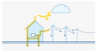
Lightning strike to the earth near the building or structure
