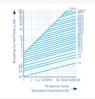
Breaking Current Characteristics Curve of "gG" Fuse Links
