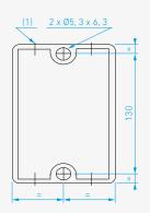
(1) Top face: 2 knock-outs for ISO20/25 cable glands or Pg16 or 16 mm conduits. Bottom face: 2 knock-outs for ISO20/25 cable glands or Pg16 or 16 mm conduits.
