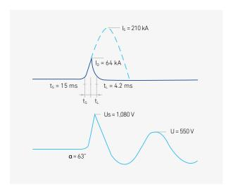
Wave curve of current limiting characteristics of fuse link Where :
