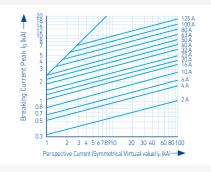
Breaking Current Characteristics Curve
