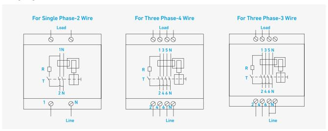
The Hyundai range of four pole RCCBs can be used to provide residual current protection in 3 phase. For 3 wire circuits (no neutral), a link from the neutral to an incoming should be made on the supply side of the RCCB, to enable the operation of the RCCB.
