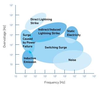
Fig 1. Various Electrical hazards
