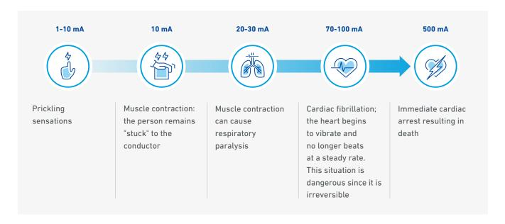
However, electrocution should not be viewed in terms of "current" alone, but in terms of "contact voltage". A person gets electrocuted by coming in contact with an object that has a different potential from his/her own. The difference in potential causes the current to flow through the body.
