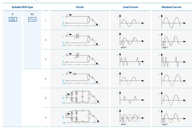
Device is suitable for electronic equipment with input current circuits 1 to 6 in below table.
